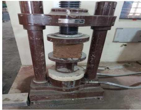
Fig 4.2 Compression strength test
