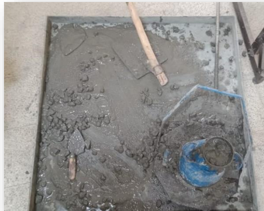
Fig 4.1 Slump cone test
